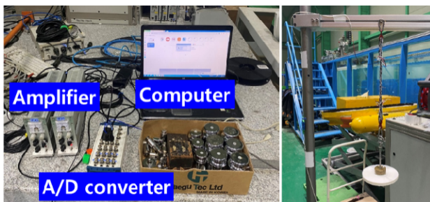
Fig. 6 Setup for the optical sensor calibration
