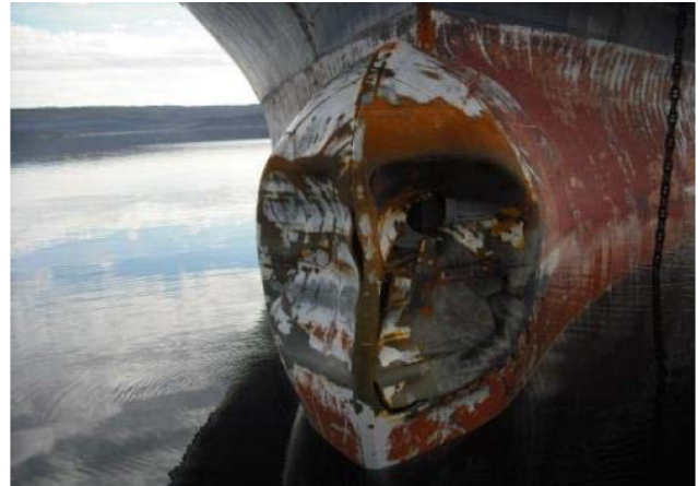
Fig. 5 Bulbous bow of a cargo vessel with a Lloyd's 100 A1 Ice Class 1A damaged in ice en route Iqaluit, Nunavut, in July (Canadian Coast Guard, 2012)
