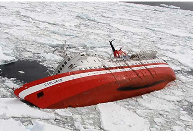
Fig. 8 The Explorer lying over its side after collision with ice wall (BBC News, 2007)
