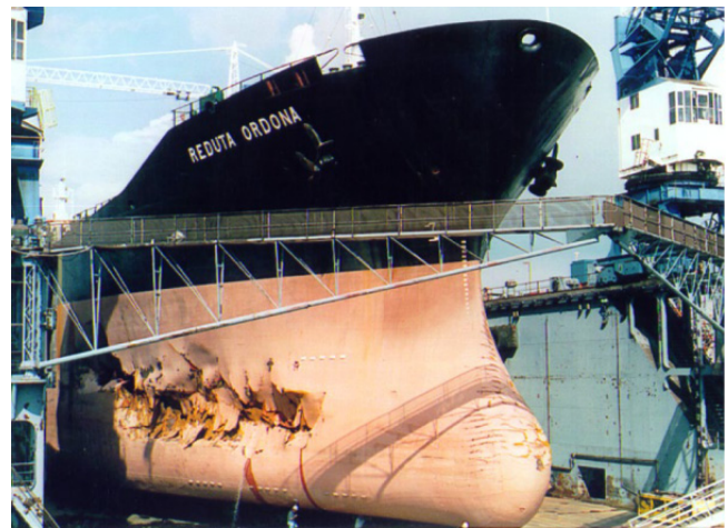
Fig. 6 Damaged side structure of bulk carrier Reduta Ordona by collision with a growler in Hudson Strait on its way from Poland to Churchill, Manitoba, July 21, 1996. Quebec City, MIL Davie shipyard (Foumler et al., 2020).
