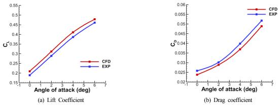
Fig. 5 Comparison of Normal hydrofoil performance between experiment and numerical simulation
