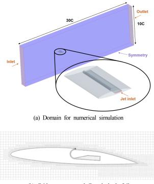
(b) Grid system around Coanda hydrofoil
