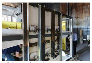
(f) String potentiometer for displacement measurement
