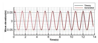
Fig. 4 Comparison of Stokes 5th order wave and generated wave  $(\lambda/L_m = 1.0, H/\lambda = 0.02)$
