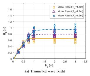
Fig. 7 Transmission characteristics at crest height R<sub>e</sub> via numerical model
