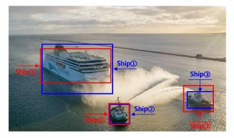
Fig. 6 Test result for the ship recognition
