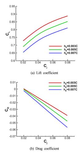
**Fig. 8** Lift and drag performance according to slit height ( $\alpha = 4^{\circ}$ )
