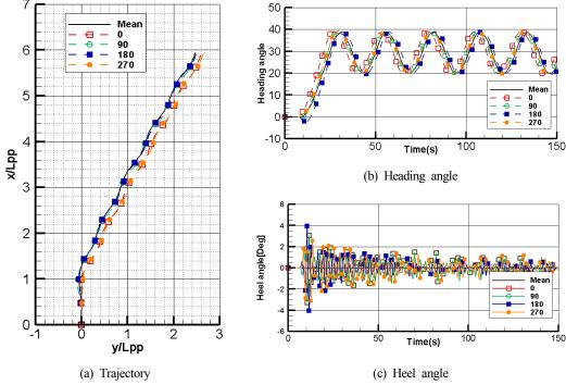
Fig. 13 Weather vaning simulation result at  $\lambda/L=1.6$
