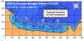
Fig. 5 Wave height distribution (without an ACR)
