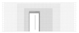
(b) Grid system around Coanda hydrofoil
