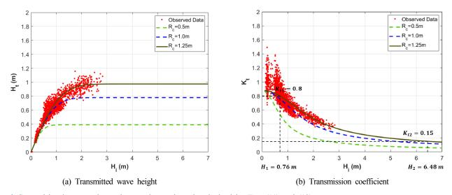
Fig. 4 Comparision between observed wave data and results obtained by Eqs. (11) and (12)
