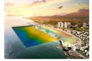
(a) Contour line of bathymatry at Bongpo beachFig. 6 Water depth at Bongpo beach and for wave model
