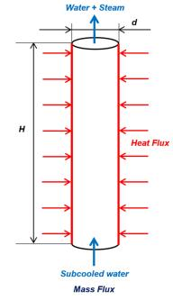
Fig. 2 Definition of the problem of flow boiling in a tube
