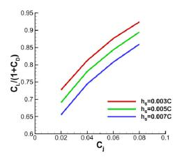
Fig. 9 Variation of lift and drag ratio according to slit height ( $\alpha = 4^{\circ}$ )
