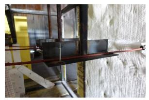
(e) Support for horizontal displacement measurementFig. 6 Measurement instrumentation for fire experiment
