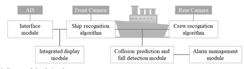
Fig. 2 Conceptual diagram of the designed system
