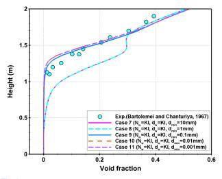
Fig. 8 Comparison of the void fraction distribution by the minimum bubble departure diameter
