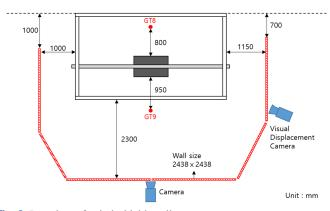
Fig. 3 Location of wind shield walls
