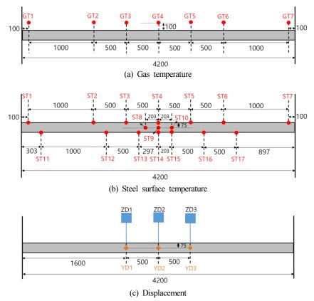
Fig. 5 Measurement positions of burner fire experiment
