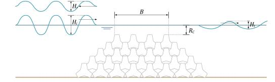
Fig. 1 Definition sketch of crest height  $R_c$ , incident wave height  $H_i$ , reflected wave height  $H_r$  and transmitted wave height  $H_i$
