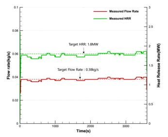
Fig. 2 Measured propane flow rate and calculated heat release rate
