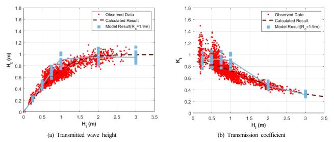
Fig. 8 Comparison of observed data, calculated, and numerical model results ( $R_c = 1.9$  m)
