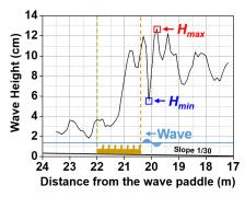
Fig. 7 Results of wave height in the physical model
