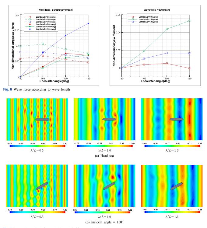
Fig. 7 Free surface distribution at head sea / incident angle 150°
