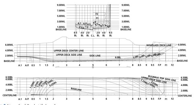
Fig. 9 Lines of a fully electrified car ferry
