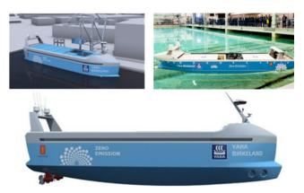
Fig. 2 Autonomous transport electric container cargo ehip (YARA) in Norway
