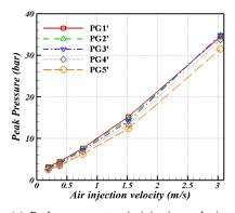
(a) Peak pressure to air injection velocityFig. 14 Peak pressure analysis in the bent pipe
