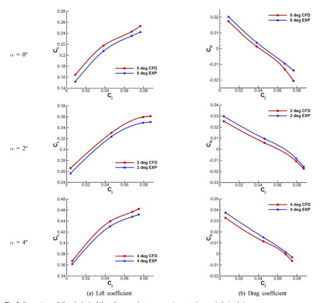
Fig. 6 Comparison of Coanda hydrofoil performance between experiment and numerical simulation
