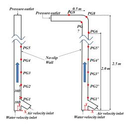
Fig. 1 Schematic image of the computational domain
