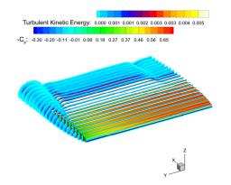
Fig. 16 Turbulent kinetic energy around the Coanda hydrofoil with 3D effect ( $\alpha = 4^{\circ}$ ,  $C_i = 0.06$ )
