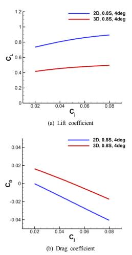
Fig. 14 Comparison of lift and drag performance between two and three dimensional ( $\alpha = 4^{\circ}$ )
