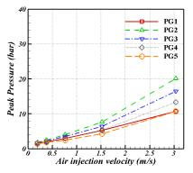
(a) Peak pressure to air injection velocityFig. 10 Peak pressure analysis in a vertical pipe
