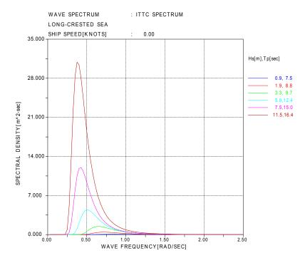
Fig. 10 Wave spectrum
