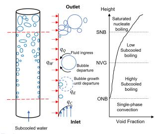
Fig. 1 Schematic diagram of the wall boiling model
