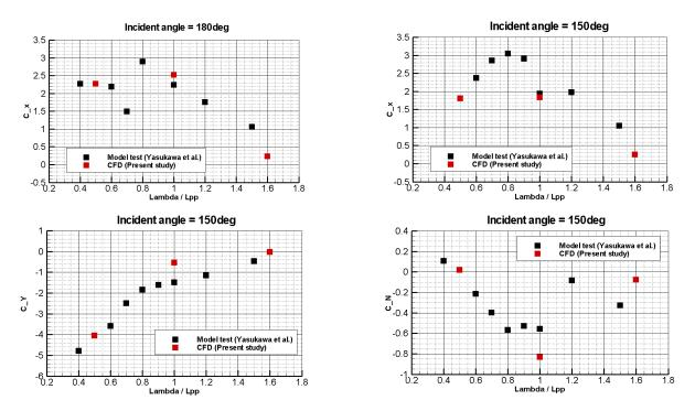
Fig. 8 Comparison of wave force based on CFD results and model test results
