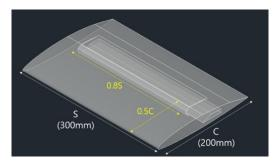
(a) Dimension of Coanda hydrofoil and jet flow range
