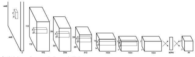
Fig. 3 YOLOv2 network structure (Redmon et al., 2016)
