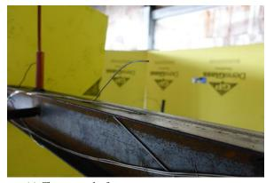
(a) Thermocouple for gas temperature measurement
