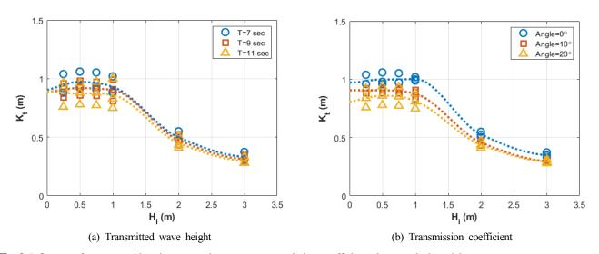
Fig. 9 Influence of wave peroid and wave angle on wave transmission coefficient via numerical model
