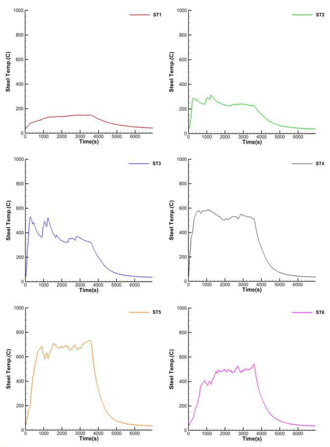
Fig. A2 Test results - steel surface temperature (continuation)
