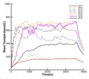
Fig. 10 Steel surface temperature results of lower flange
