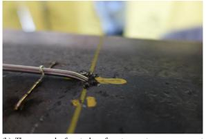
(b) Thermocouple for steel surface temperature measurement
