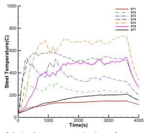
Fig. 9 Steel surface temperature results of upper flange
