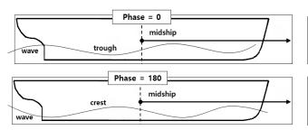
Fig. 9 Wave initial condition - encountered wave phase at midship
