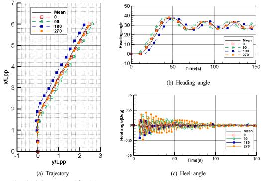
Fig. 11 Weather vaning simulation result at  $\lambda/L=0.5$
