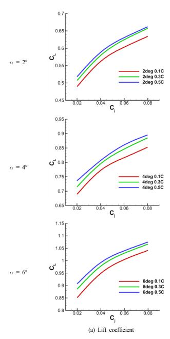
Fig. 11 Lift and drag performance according to slit position
