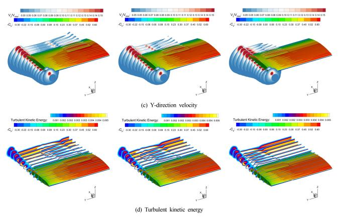
Fig. 22 Flow characteristics around the Coanda hydrofoil with various slit range ( $\alpha = 4^{\circ}$ ,  $C_i = 0.06$ )
