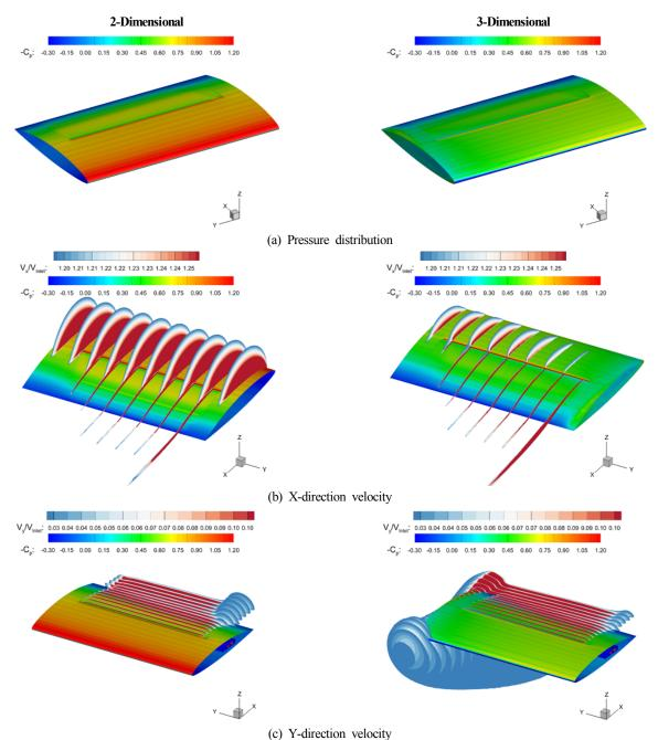
Fig. 15 Flow characteristics around the Coanda hydrofoil ( $\alpha = 4^\circ$ ,  $C_i = 0.06$ )
