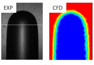
(a) Snapshot Fig. 5 The experimental and numerical shape of Taylor bubble
