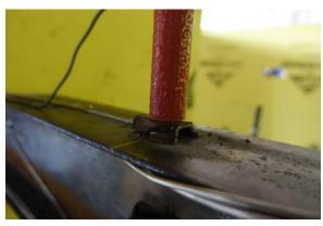
(c) Instrumentation for vertical displacement measurement
