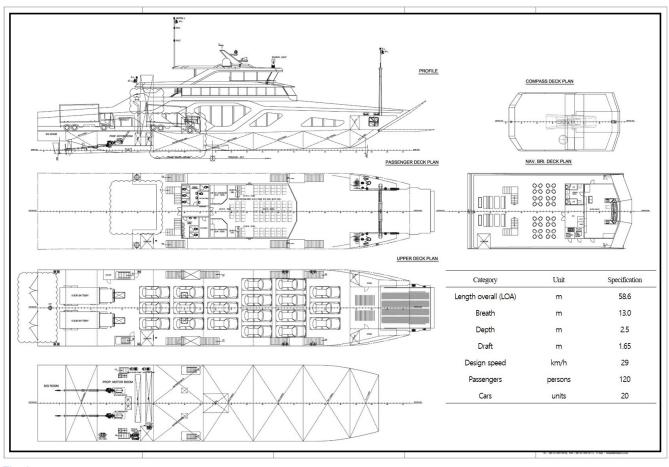
Fig. 8 General arrangement of a fully electrified car ferry
