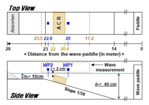
Fig. 6 Experimental design for the physical model test
