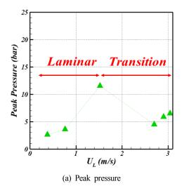
Fig. 17 Comparison of the peak pressures with various water velocity
