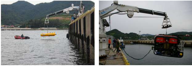
Fig. 14 Launch and recovery of ISiMI 6000 AUV and Hemire ROV using a crane in a port
