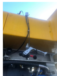
Damaged URI-T frame
